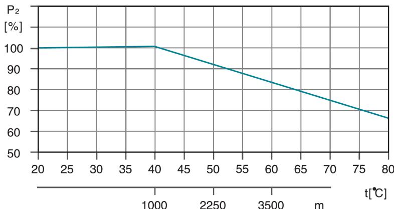
For example, when the pump is installed at an altitude of 3500 meters, P2 will decrease by 88%. And when the ambient temperature is 70 ° C, P2 will decrease by 78%.
